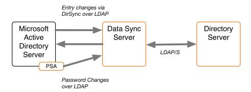
The PSA supports failover between servers. It caches the hashed password changes in a local database until it can be guaranteed that all PingDataSync Servers in the topology have received them. The failover features enable any or all of the PingDataSync Servers to be taken offline without losing any password changes from Active Directory.
