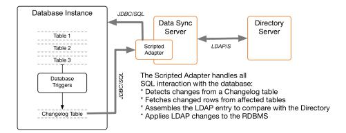
PingDataSync Server synchronizes data between a directory server and an RDBMS system with a Server SDK extension. PingDataSync Server provides multiple configuration options, such as advanced filtering (fractional and subtree), attribute and DN mappings, transformations, correlations, and configurable logging.
