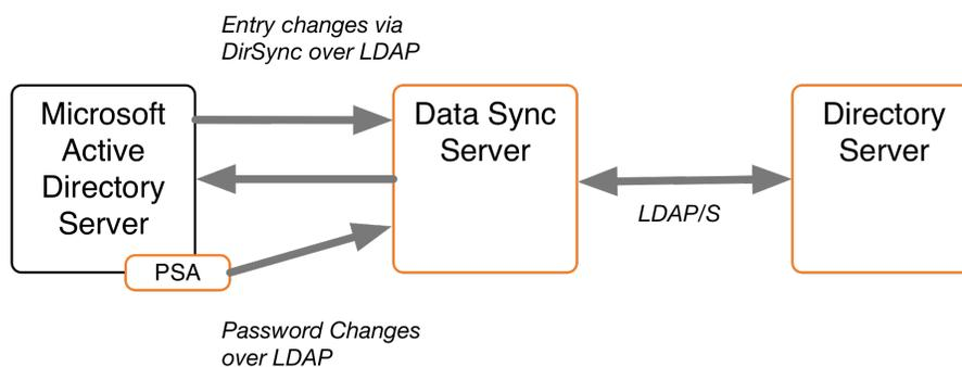
The PSA supports failover between servers. It caches the hashed password changes in a local database until it can be guaranteed that all PingDataSync Servers in the topology have received them. The failover features enable any or all of the PingDataSync Servers to be taken offline without losing any password changes from Active Directory.
