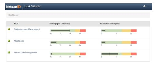
**sla-viewer-details** – Displays SLA Viewer data and additional charts for response time and time ranges from the sla-viewer dashboard. Data can be viewed per server and includes server details.
